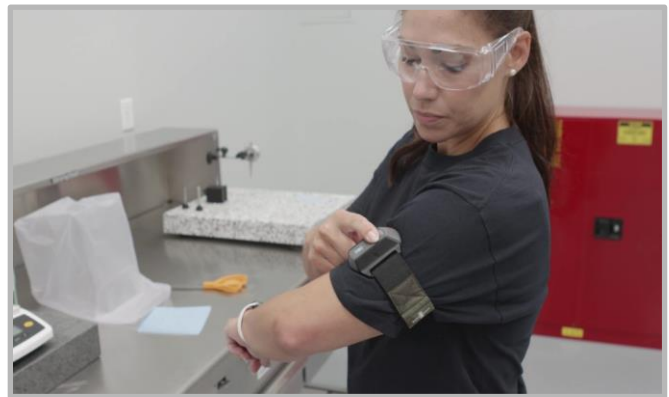
MākuSafe's signature armband, equipped with sensors for ambient light, air quality, noise, air pressure, humidity, and temperature 15
